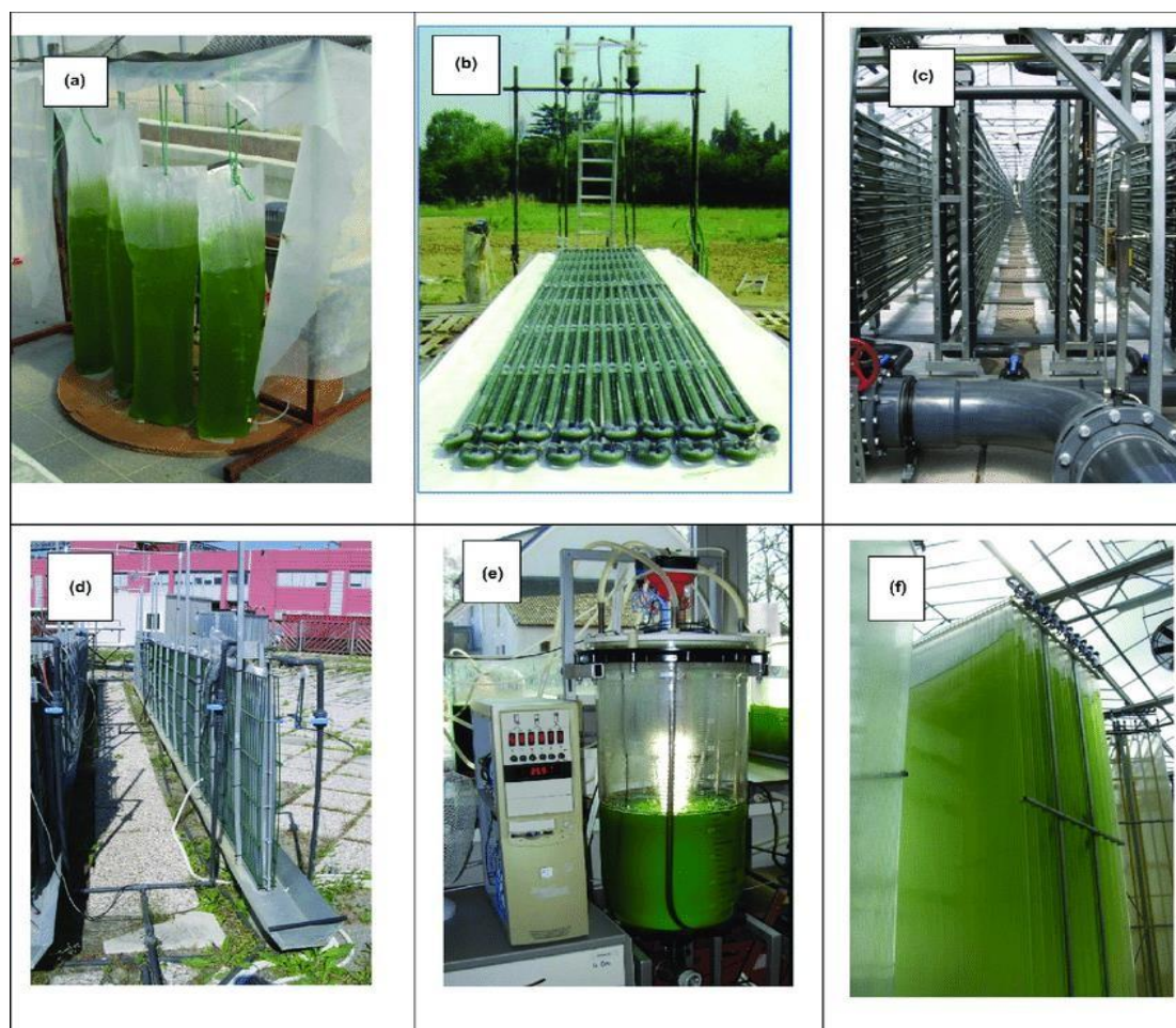
Figure 4: Closed or semi-closed photobioreactors for microbial culture that can be grown up to bigger manufacturing plants [14] .
